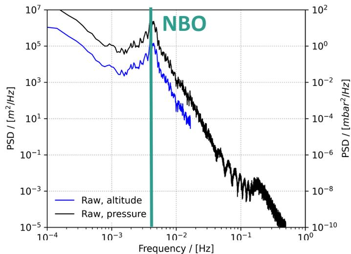
Balloons position determined by buoyancy, wind forces, gravity. Presence of a **Neutral Buoyancy Oscillation** = balloon normal mode.
