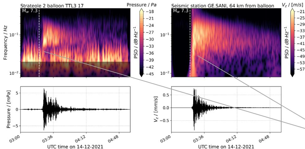
Good agreement between seismic ground sensors and airborne infrasound recordings
